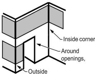
Outside corners should be cut at a 45 degree angle. Inside corners should have an overlap of 3 mm.
