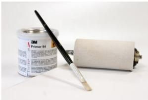
Low surface energy (hard to adhere): has to be primed completely.
