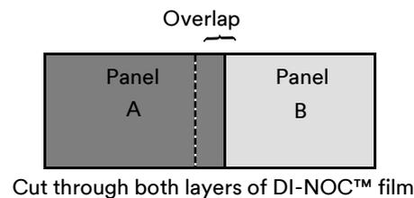
2. On the film side where the seam will be, leave 2.5 cm of the liner on the side of Panel A.
